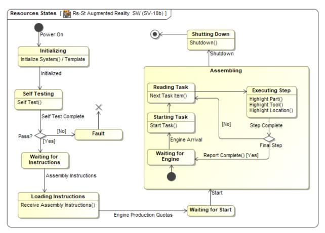
Figure 17. Augmented Reality Assembly State Diagram
