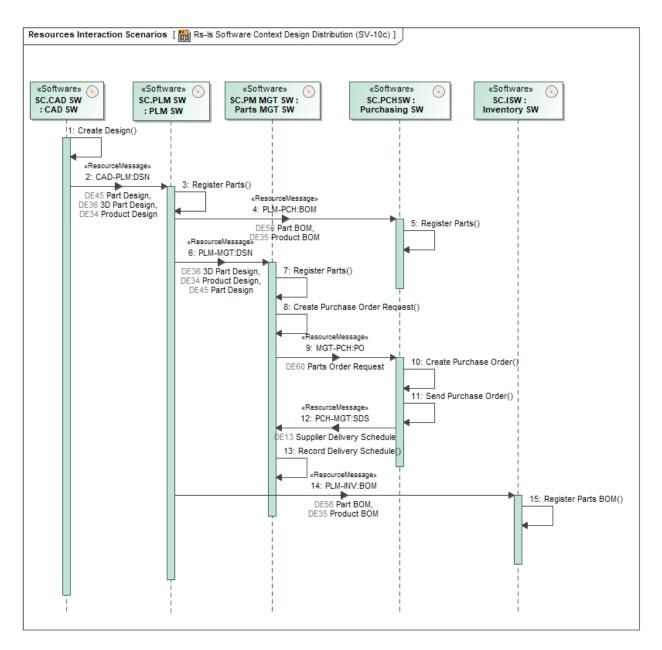
Figure 13. Design and Parts Distribution Sequence
