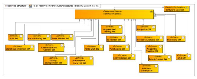
Figure 8. Aggregating the Software into a Virtual Architecture
