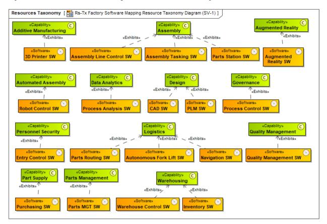
Figure 6. Mapping the Capabilities to the Implementing Software
