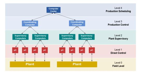
Figure 1. Hierarchical Factory Control System <u>https://commons.wikimedia.org/wiki/File:Func-</u> tional\_levels\_of\_a\_Distributed\_Control\_System.svg
